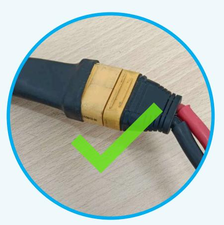
Ensure tightly secured connection
